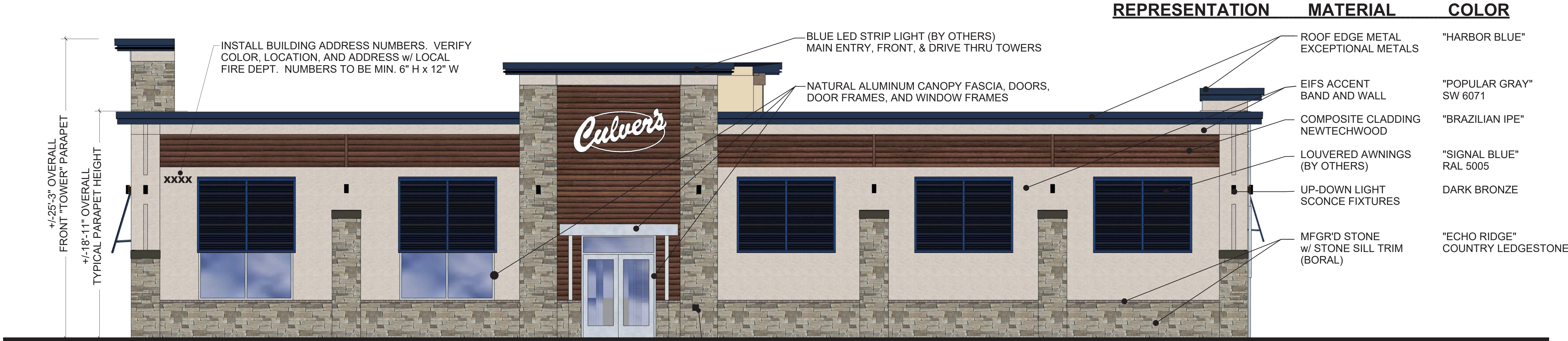
MAIN ENTRY ELEVATION
