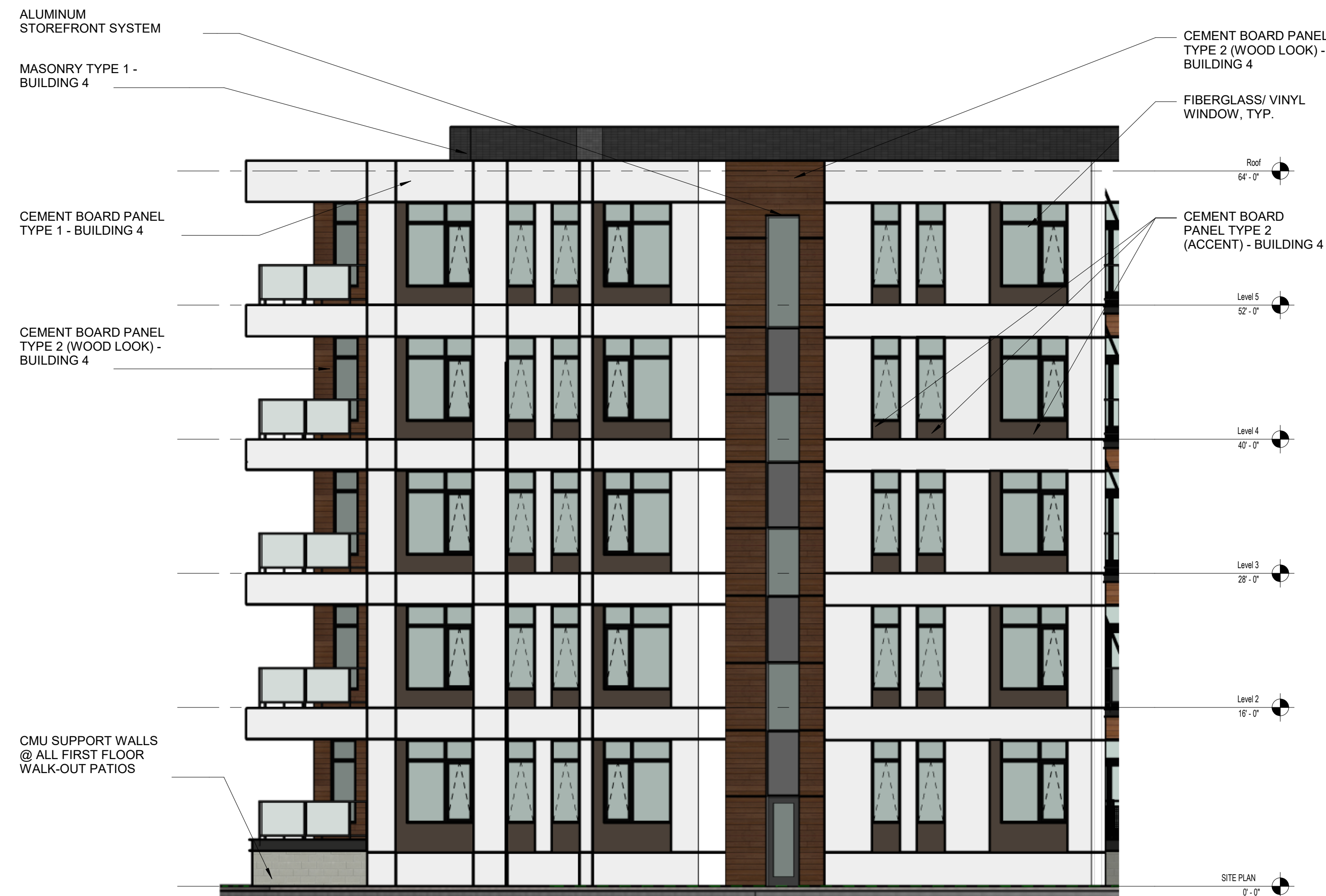
1 BUILDING ELEVATION (SOUTHEAST) SCALE: 1/8" = 1'-0"
