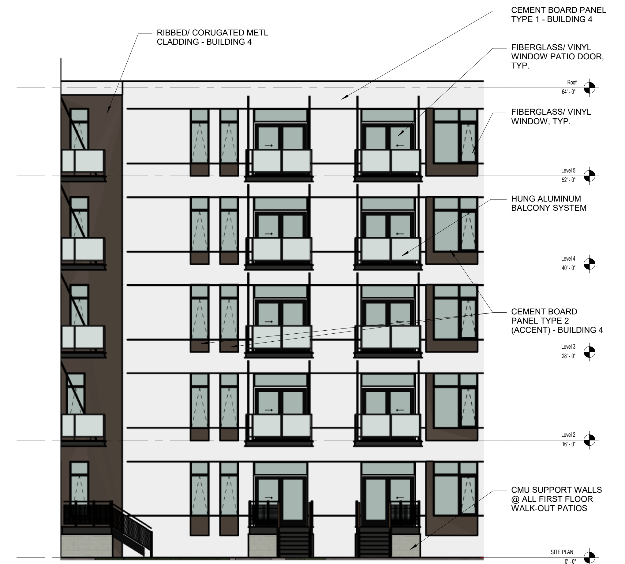
3 BUILDING ELEVATION (SOUTH) SCALE: 1/8" = 1'-0"
