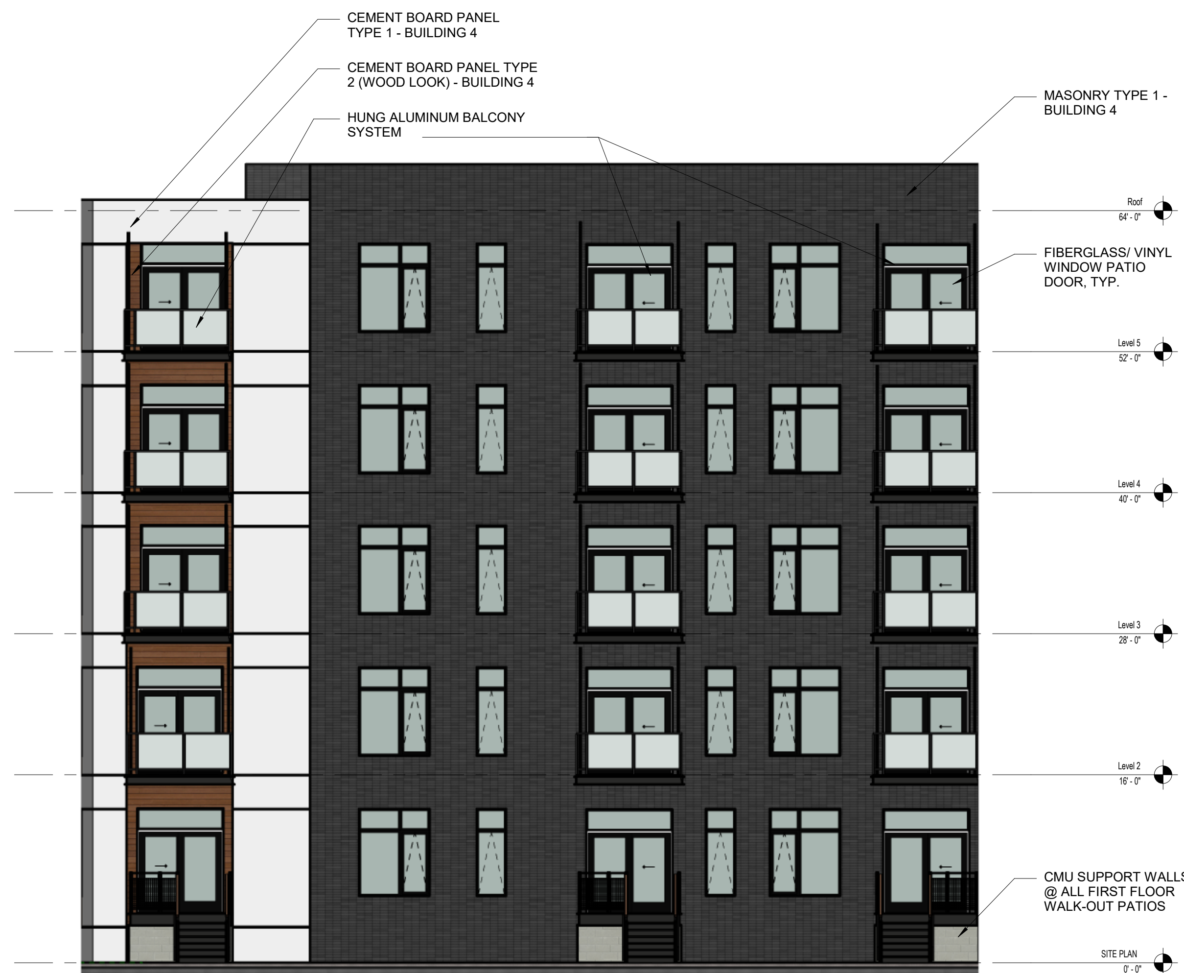
2 BUILDING ELEVATION (EAST) SCALE: 1/8" = 1'-0"
